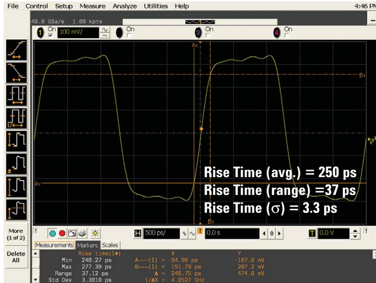
Figure 15a: 400-MHz clock captured on an Agilent Infiniium DS080304B 3-GHz oscilloscope sampling at 40 GSa/s
