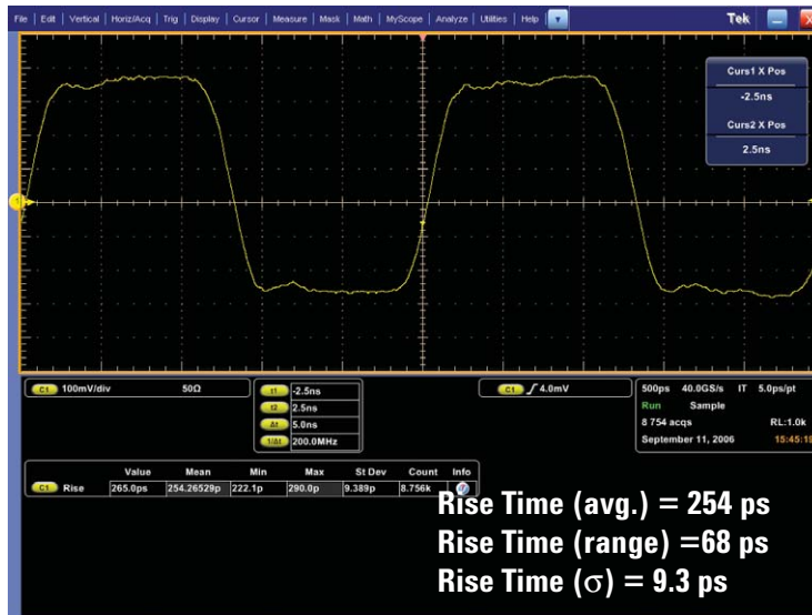
Figure 15b: 400-MHz clock captured on a Tektronix DP07254 2.5-GHz oscilloscope sampling at 40 GSa/s
