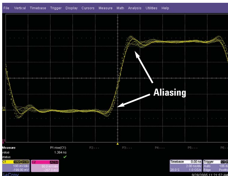
Figure 4: 500-MHz bandwidth scope sampling at 1 GSa/s produces aliased edges
