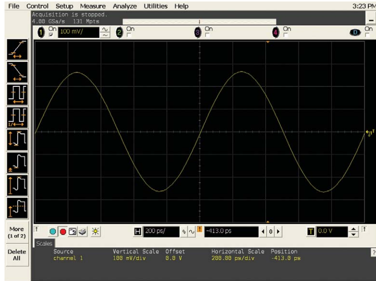
Figure 11a: 1-GHz sine wave captured on an Agilent MSO8104A 1-GHz bandwidth oscilloscope sampling at 4 GSa/s
