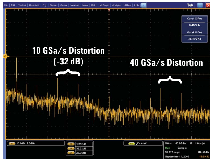
Figure 14b: FFT analysis of 2.5-GHz sine wave captured on a Tektronix DPO7254 sampling at 40 GSa/s
